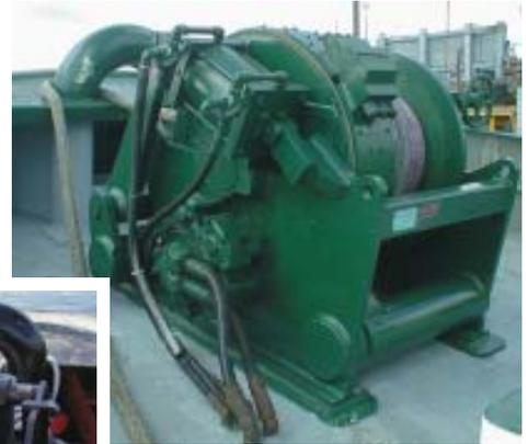
**Class II Markey "Render/Recover"® Winches** include Markey-pioneered adjustable automatic "constant tension" inhaul, up to the power limits of the winch drive, for all tethered operations. Tugs outfitted with Class II winches can safely maneuver through day-long escorts while the winch automatically adjusts scope to maintain preset line tension. Available in hydraulic or electric versions.
