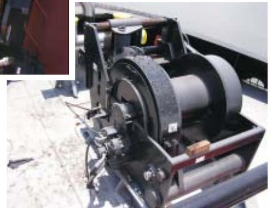
**Class III "ARR" Hawser Winches** are ultra-high performance soft line winches for indirect towing and improved shock load control in extreme sea ways. Below deck all-electric drives and water cooled multi-disc slip-brakes ensure secure load control at full rated tug speeds and to 250% of static bollard pull. Class III designs are available with remote trouble shooting and performance monitoring via the world wide web.
