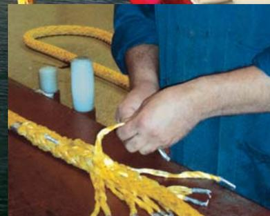
Developments in maritime rope over the past 50 years have focused on new synthetic yarns to produce stronger and lighter ropes. Meanwhile the construction of the soft 'eye' splice at the end of the rope for mooring and towing operations has remained largely unchanged, until now. Lankhorst Ropes has drawn on over 200 years experience in maritime ropes to develop new rope splice technology.
