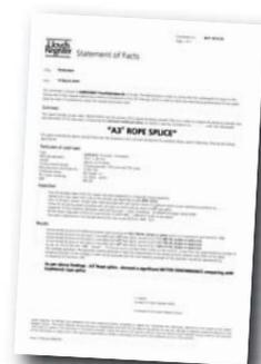
The Tipto-Winch Line with a breaking force of 682 kN showed a breaking force of 785 kN for the A3® splice. Further development of the new splice with other synthetic yarns is now in progress.
