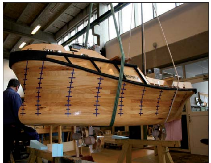
Figure 6: The model for tank tests.
