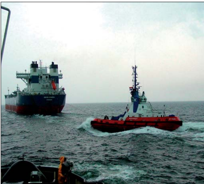
Figure 2: Rotor tug Magic in the escort mode when stern first.
