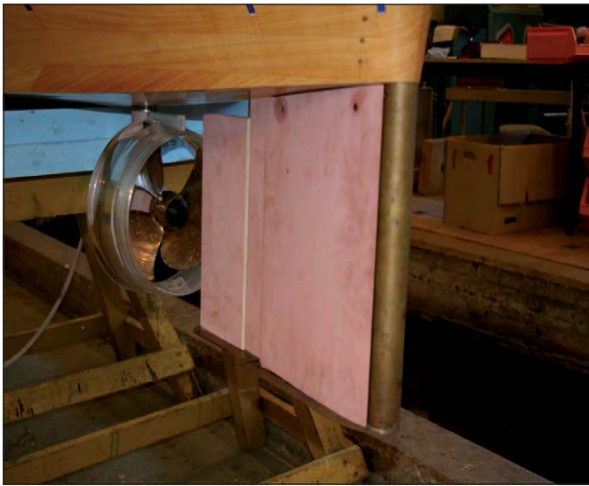
Figure 7: Aft end of the model with Z-drive, skeg and flap.
