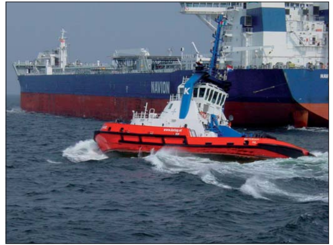
Figure 3: Rotor tug Magic in the escort mode when bow first.
