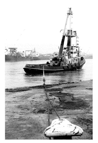
The achieved traction force is described as the "Continuous Bollard Pull" and has to differentiated from the so called "Static Bollard Pull".
