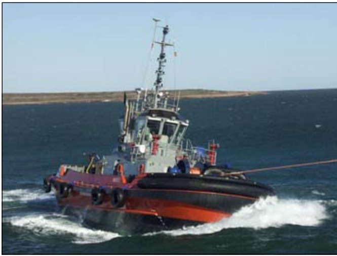
Figure 3: Typical escort tug operational attitude (courtesy of Robert Allen Associates).
