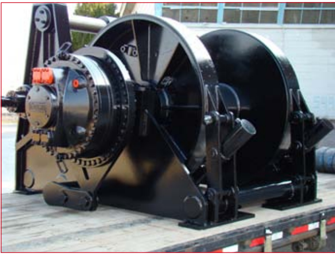
Figure 10: Escort tug winch (courtesy of JonRie).
