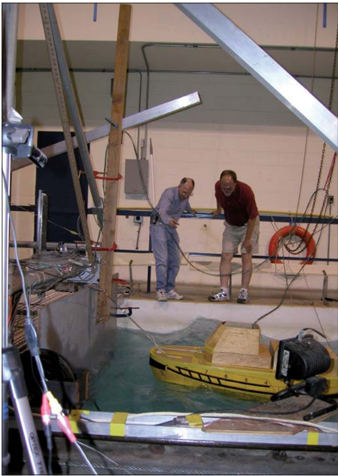
Figure 2: Model test of dynamic sea hawsers
