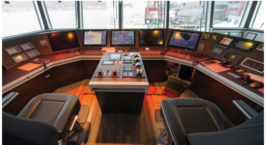
▲ Maersk Master is the first of the Starfish series to be fitted with the integrated bridge system
