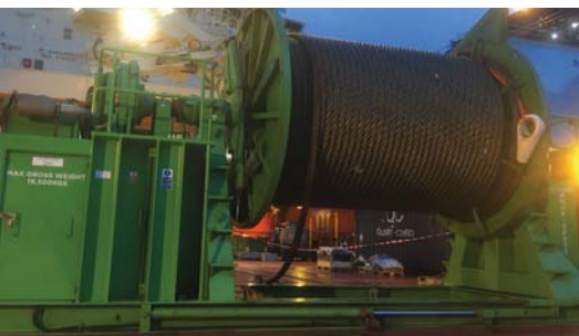
◀ A Gaylin Group 250-ton capacity back tension spooling machine
