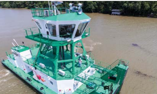
◀ Estaleiro Rio Maguari's 45-tonne bollard pull tug Waldemaro Schmidt , top, designed by Interocean for use on Brazil's inland waterways. Bottom, the company's latest 1,200hp river pushboat, designed by Canada's Robert Allan Ltd
