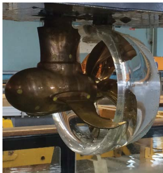
◀ The new VarioDuct SDV45 nozzle, shown with Rudderpropeller
