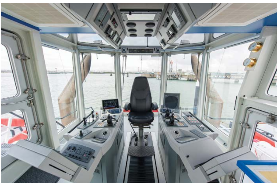
▲ AlphaBridge on the Robert Allan Ltd designed hybrid RotorTug RT Evolution built by Damen Shipyards Hardinxveld
