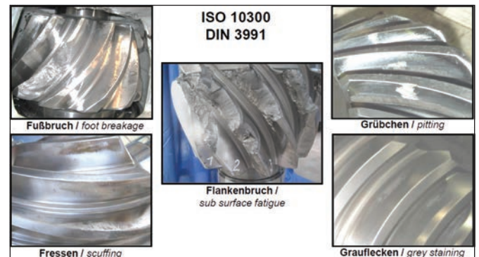
Figure 13: Typical types of gear damage of a bevel gear set (Image: Schottel)
