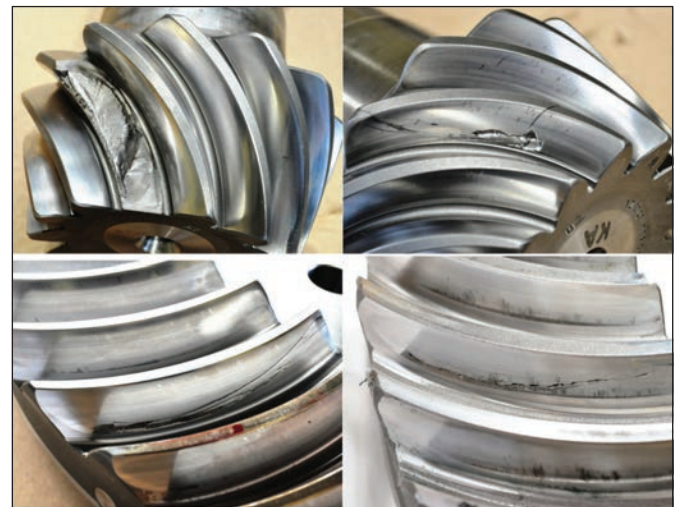
Figure 27: Intentionally produced sub-surface fatigue damage (Schottel Hellbox) (Image: Schottel, Potts')
