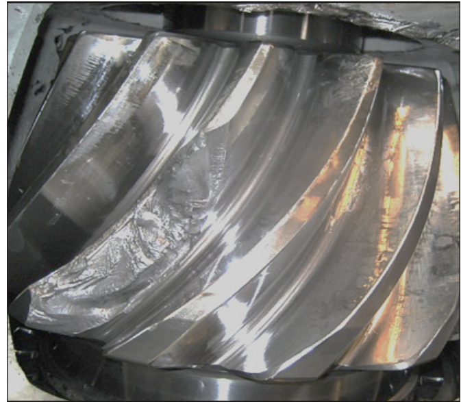
Figure 22: Foot breakage of a bevel gear toothing (Image: Schottel)
