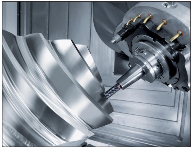
Figure 5: Alternative machining using the 5-axis milling process (Image: Bierens)
