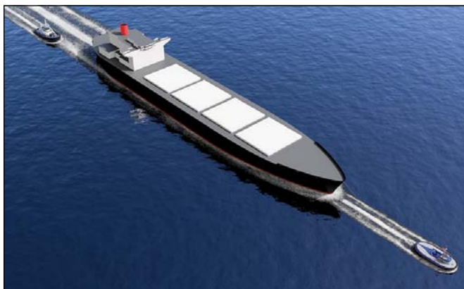
Figure 15: Moving with the ship with RAMora in centre lead position, slack line
