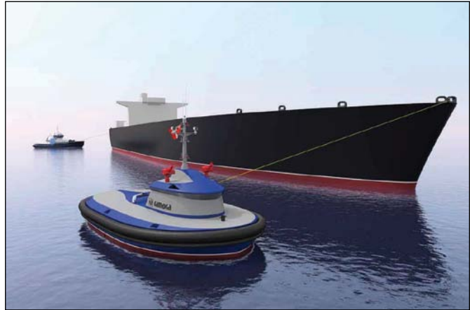
Figure 8: RAmora working in tandem with conventional tug centre lead forward position
