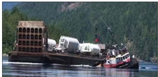
Figure 6: Girthing of tug North Arm Venture in strong current
